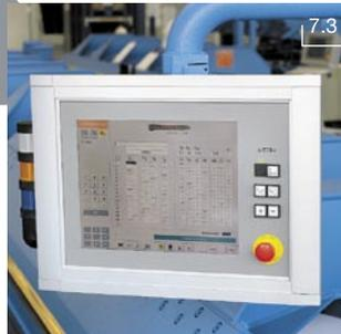
**7.3 CNC5000 touchscreen control system** with 17" TFT colour display. The control system operates with a Windows-based Pentium processor with automatic rear stop and the possibility of controlling a tapered rear stop. Included in the scope of delivery is a CAD drawing program (see our full brochure for more detailed information).
